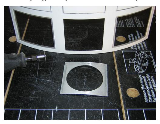
The skins are not the only thing requiring work to accommodate the power couplers. Due to the new power coupler frame, I must Dremel out a larger area in the frame as well. I only had time for the front power coupler area today, I hope to use the router to route out the rear power coupler area tomorrow.
