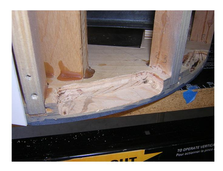
While the skirt was off, I decided to go back with white silicone, and fill in some visible seams where the ribs are attached on the skirt.
