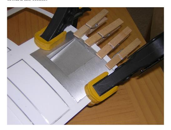
Following a tip from Doug Dixon on the board, I obtained a plastic template sheet to use as a cover for the front and rear Processor Status Indicators (PSIs). I won't know how good these work until I have the PSIs with LEDs installed, but for now they are covering up those annoying holes. I cut two layers and used masking tape to attach them to the inside of the dome.
