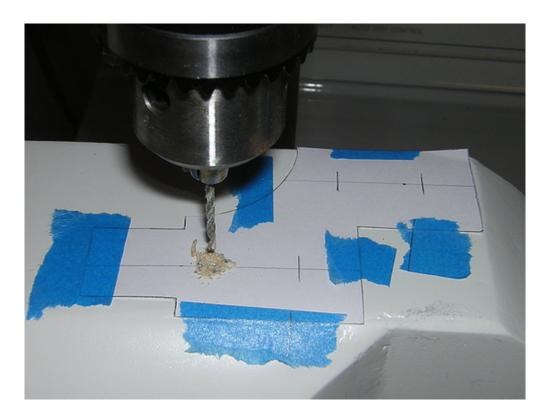
After drilling the legs, I used the same paper template and taped it to the back of the resin ankle detail pieces. I drilled through these one at a time, again about 1/4" deep. Then I used a hacksaw to cut 16 toothpicks to size. (That was fun...)
