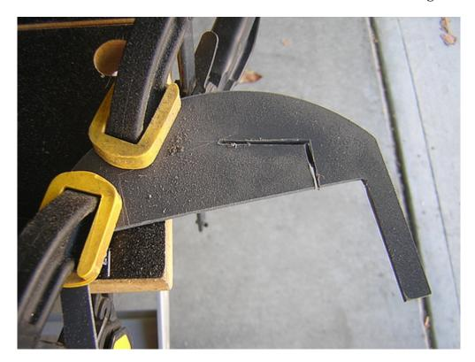
I used the Dremel drum sander to round out the area where the leg strut shaft will go.
