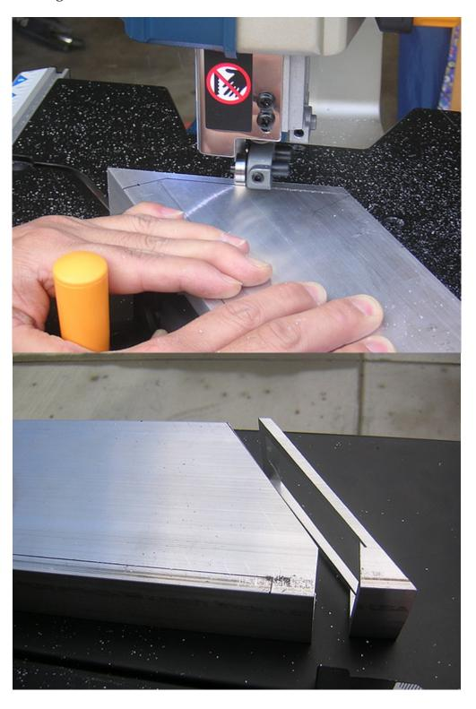
The band saw did a very good job of cutting through the aluminum 2x4, even on some of the longer cuts.
