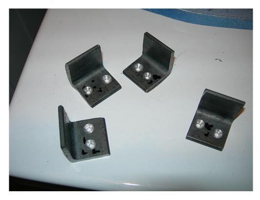
I used a hammer to put a slight bend in the L-bracket, so that the curve of the door won't bump into the bracket.
