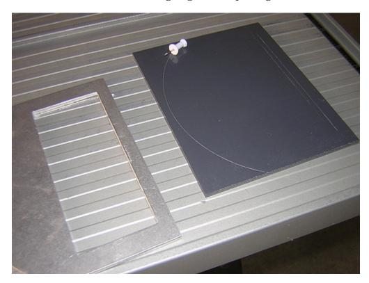
After that, I rough-cut the curve using the Dremel cut-off wheel attachment. This was like a knife through butter, but don't breath the fumes!
