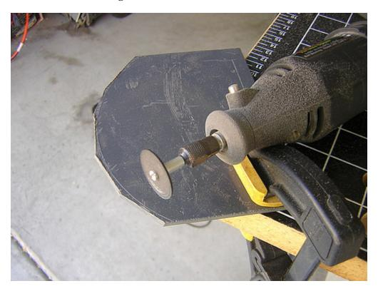
I cleaned up the curve with the Dremel drum sander attachment.
