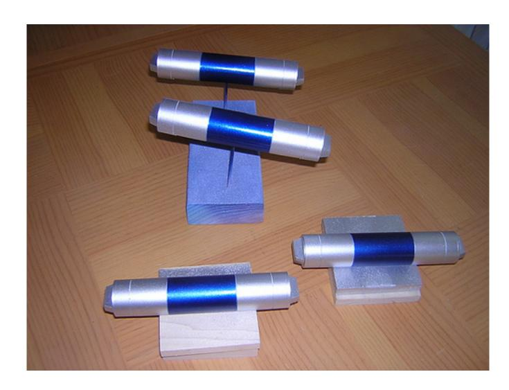
I also prepped the ankle cylinder holders for primer/painting by drilling a hole on the holder side, so they can sit upside-down on top of the same rods that the cylinders were mounted on. Hopefully I'll start the process tomorrow.
