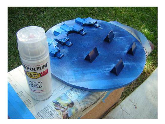
Finally, I touched up the holes where the buttons and hydraulics live in the horseshoes. I didn't get complete coverage with the spray paint, so I sprayed some of the same paint into a pie tin, and used a small paint brush to touch up those areas.
