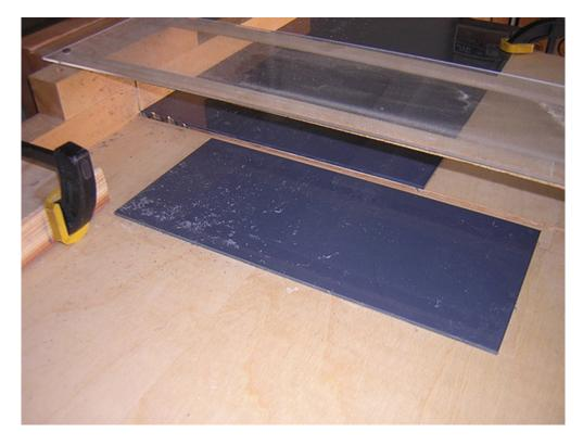
Next, I traced the outline of the bracket shape onto the PVC, using a pin and an aluminum bracket that I'm not going to end up using on this droid.
