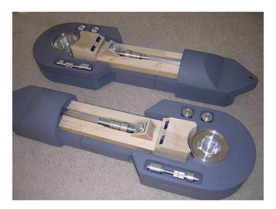
I also did some minimal work related to the utility arms. These are to be held in by a fixed piece of MDF, and a screwed-down piece of aluminum stock. Each of these pieces will have half of a circle cut out of them, supporting the rod that goes though the pivot point in the utility arms. I cut eight pieces of aluminum total, but I really only need four. I figured it couldn't hurt to cut extras, especially since some of them didn't turn out so great.
