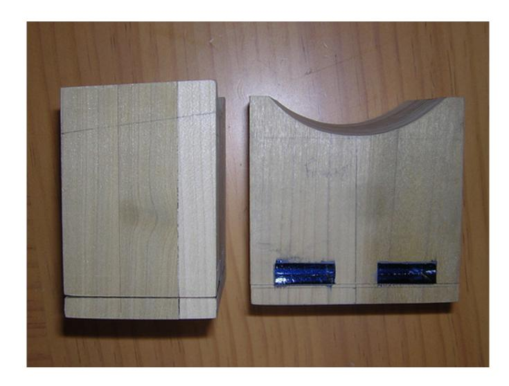
I still need to route a curve out of the bottom-front corner, and cut 3 degrees off the front face of the booster cover tops, then the booster cover tops will be pretty much done (except painting and adding mounting screws).
