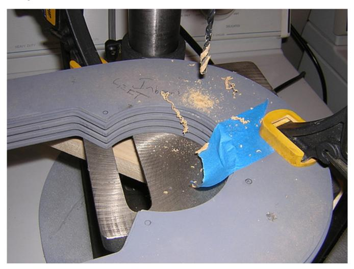
I then took the shim layer, and taped it down (opposite side up) onto the leg. Lining up the drill bit with the holes that I had just drilled into the shim layer, I drilled matching holes into the outer face of the leg. As each hole was drilled, I placed a #8 screw (head cut off) into the hole, to secure the horseshoe into the leg and keep it from moving.
