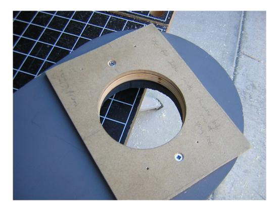
Once I unscrewed the template, I test fitted the hub in the leg. It fit pretty well, so I'm happy with it. More important, the hole for the hub is exactly centered in the horseshoe opening, which is what I was really stressing over.
