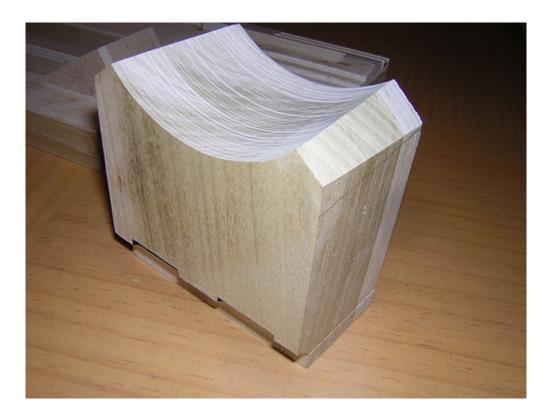
The last item of business for the day was routing the grooves in the main part of the booster covers. I set up the fence and stop accordingly, and ran the booster covers through the router four times each (once for each groove).
