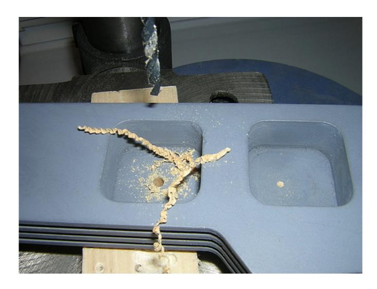
For the shoulder hydraulics, I attached a piece of tape (same width and length as the hydraulic) to the back of the part, and then screwed a screw into each of the two holes in the back, making corresponding holes in the tape. Then I took the tape, centered it properly into the slot in the horseshoes, and used that as a guide for drilling.
