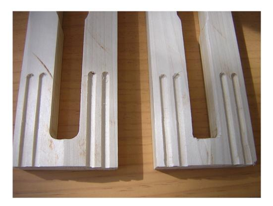
The little bit of waviness at the bottoms will go away later on, when I chop the bottoms of the booster covers off to open up the "tuning fork." I still need to cut a groove around the main part of the booster covers too, but I'll wait until I know how the booster covers are mounted, so I can match the existing grooves on the legs.
