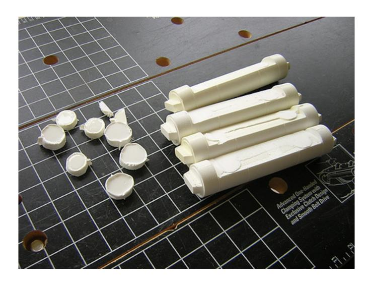
After that, I took a shot at cutting out the groove in the ankles. I drilled a 1/8" hole in each end of the groove (the blueprints don't specify the height of the groove, only the 1.875" width). Then I used the Dremel with the cutoff wheel attachment to cut the groove.
