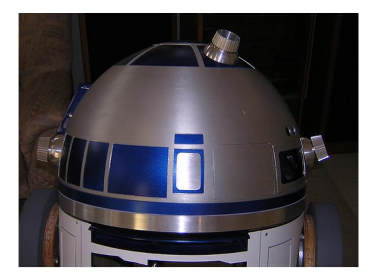
Finally, I painted black the outward facing sides of the paddles that hold the octagon ports in place. Once they were dry, I screwed them into the frame, completing the octagon port portion of the build.
