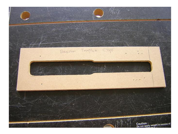
I rough-cut four booster cover layers. Before routing them all down to size, I decided to do what I did with the horseshoes. That is, I'm routing one layer down to size using the MDF template, but I'm leaving the other layer rough-cut until after the two layers are glued together. Then I'll come back with the router and route the second layer down to size, using the first layer that is glued to it.
