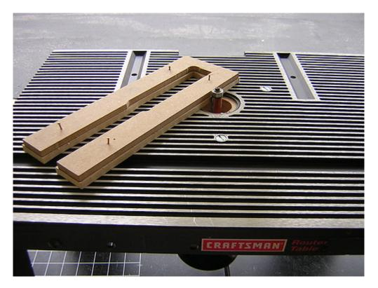
Mike suggested that I might want to close the "tuning fork" at the bottom, so the two ends would stay separated from each other by a constant distance while woodworking. So I took the cloned Senna template and made another clone, this time with the bottom ends still connected. This way the two "legs" won't have a tendency to bow as I work with the template and its resultant cuts. Later I can chop off the bottom and open up the tuning fork on the final pieces.
