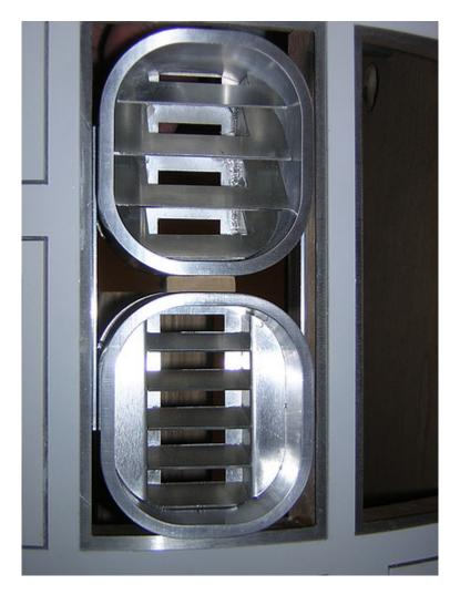
Finally, I gouged out spots on the wooden frame base plate where the coin returns will go, and I JB Welded the coin returns. I remember dreading these earlier, but they didn't end up being a complete disaster after all (although I still need to attach them to the skins...).
