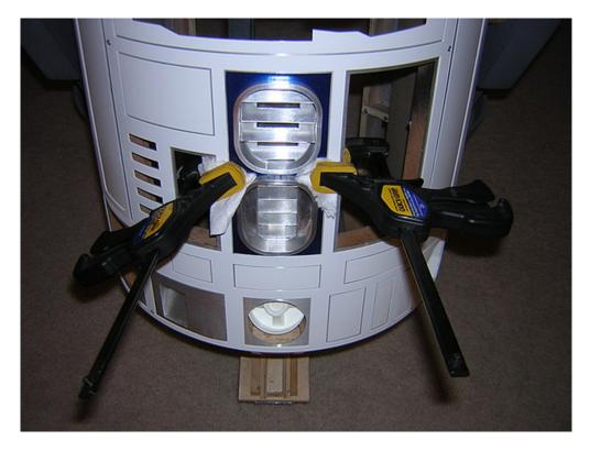
For fun, I used blue tape to secure the front octagon port into the body from behind, to see how it looks now that the latticework has been cut. Obviously I still need to paint this part.
