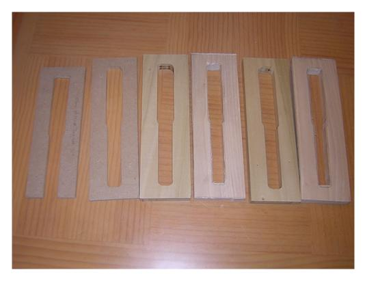
Finally, I glued the rough-cut layers to the properly-sized layers for each booster cover.
