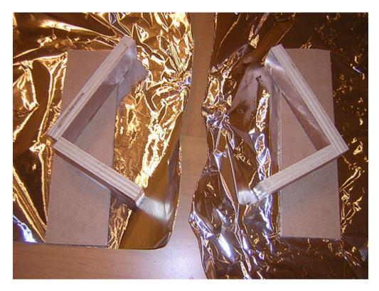
Finally, I decided to sand the backs off the octagon ports so that the latticework can show, like on the real R2 (and per the blueprints). I sanded until the resin was practically transparent, and then used an X-acto knife to finish the job.
