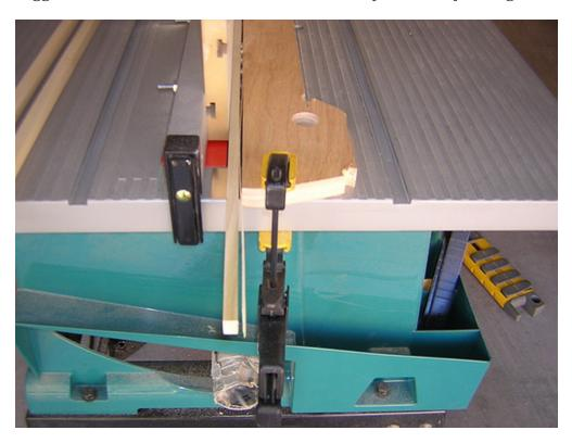
Next I cut the steep angle that rests up against the bottom of the skirt:
