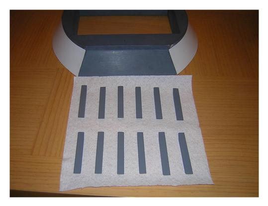
I just need to glue the ribs on and route them down to size. May need to sand the inboard parts of the ribs to make them fit the skirt snugly in places too.
