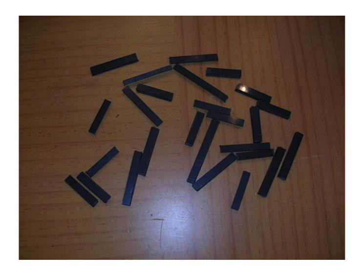
I also sanded the backing plates of the side vents and wiped them down with acetone, in preparation for painting.
