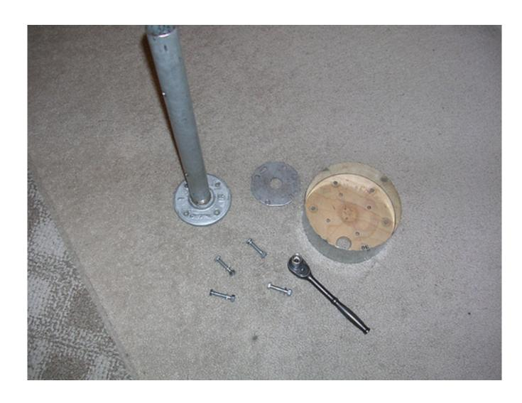
Next, I marked and drilled the backing plate.
