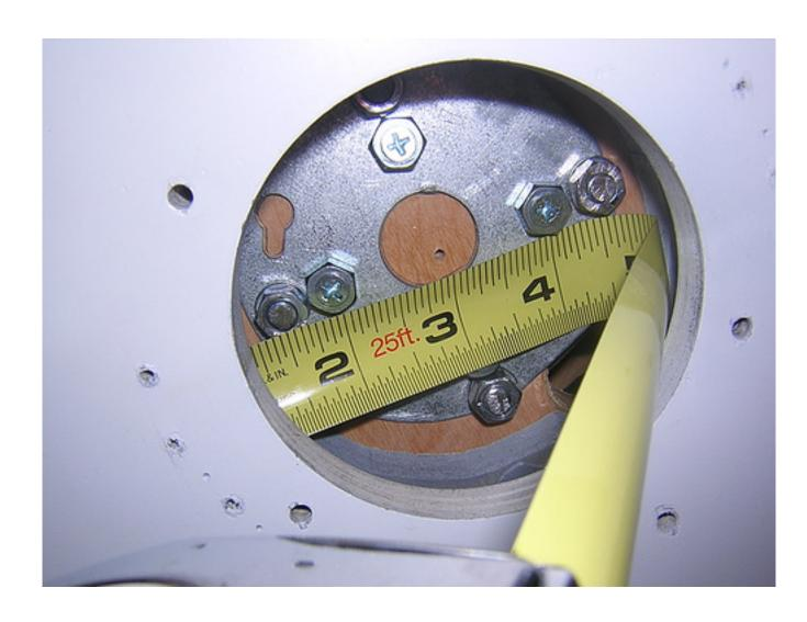
I marked the location on the shoulder hubs where the magnets should go, and drilled the holes for them.  $\,$
