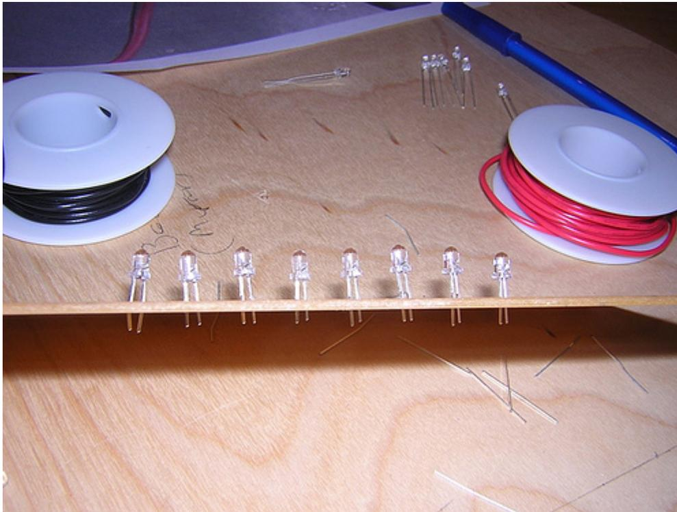
The PIC flasher circuit has a common connection for all the anodes. Being the lazy bum that I am, I just stitched the anodes together by soldering the left-over sections of the trimmed LED legs. I tested each individual LED after I was done with the whole row, and they each blinked properly. So even though the solder job is ugly, it works.
