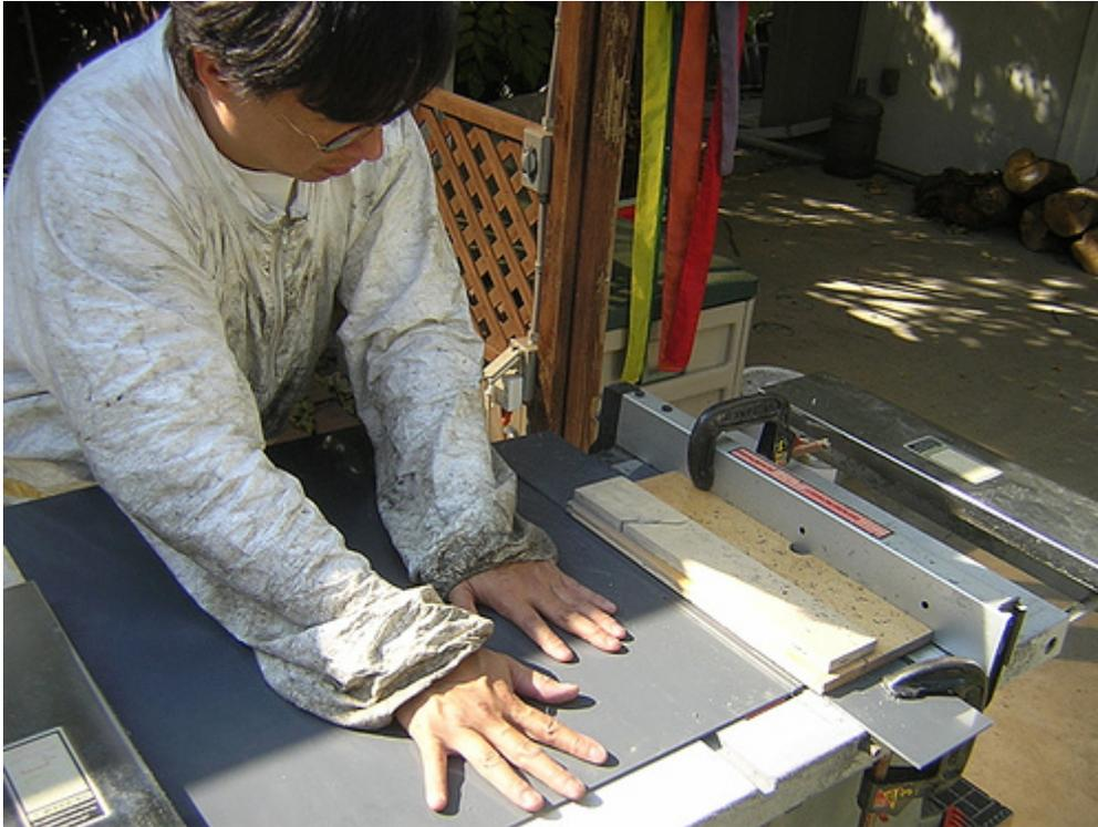
Thirty-six more strips were cut (plus twelve backing strips, plus a few extras). The blueprints show different angles for the outer feet (12 degrees) vs. the center foot (18 degrees). We decided to go with what Mike did on his first droid, and cut all the strips at 12 degrees.
