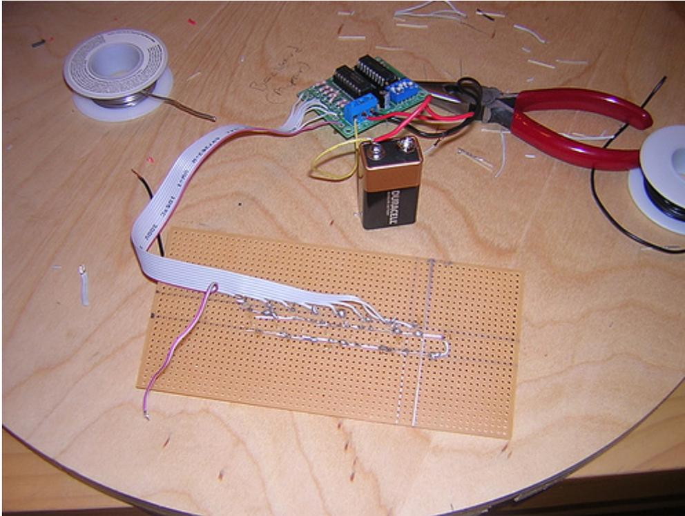
Looks like the crude soldering job was good enough to work. I'll start criss-crossing some of the LEDs' cathodes to finish the bottom row tomorrow.
