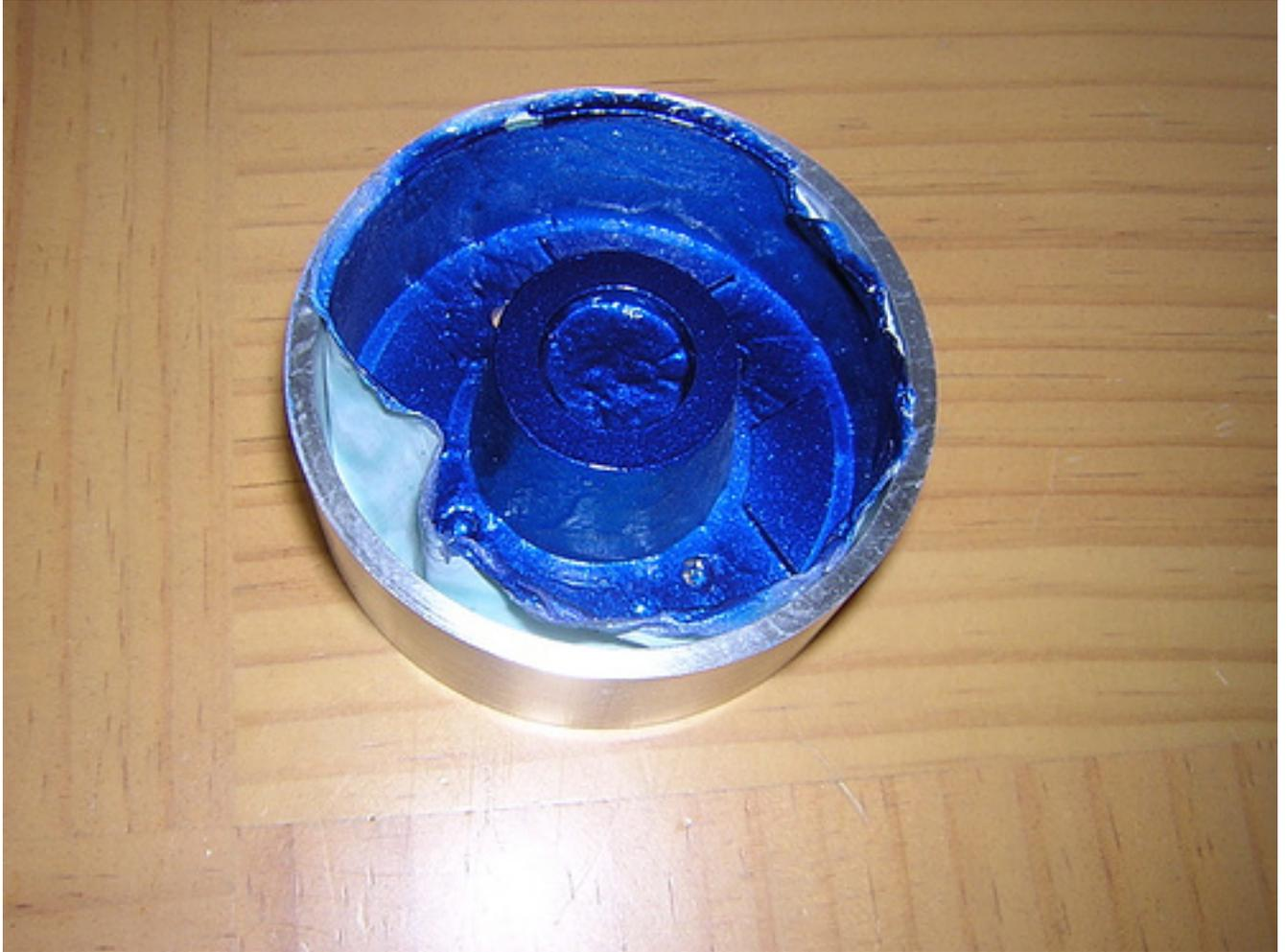
After getting the bulk of the mask out successfully, I used an Xacto knife to trim the edges of the mask on both the main power coupler body, and the power coupler frame.
