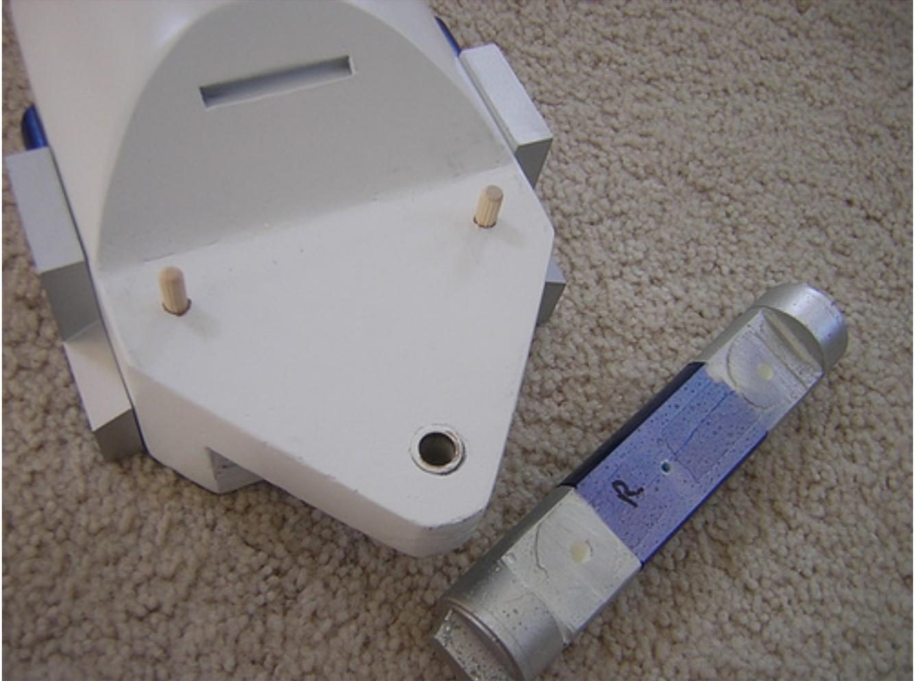
I used silicone to attach the cylinder wedges and holders.
